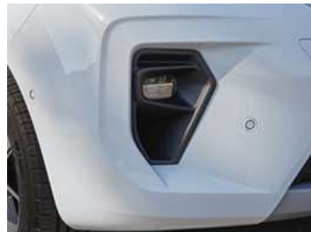
LED front fog lights with cornering technology [1]
